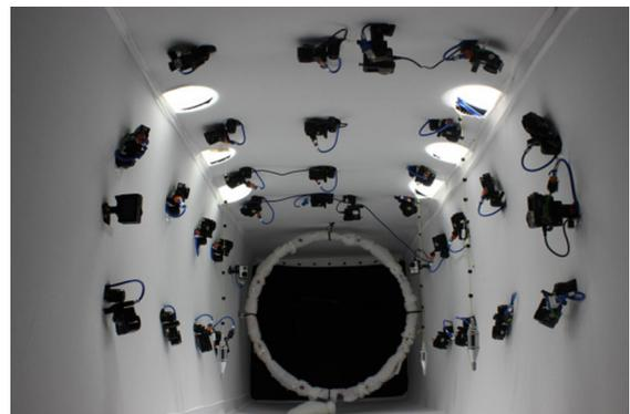
**Fig. 2** The tunnel equipped with an array of GoPro cameras for recording the flight motion of bats
